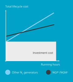
With an air factor\* of 1.8 (at 95%) to 5.5 (at 99.999%) and a special cycle time modulation algorithm, the running cost of the new NGP $^+$  can be reduced by 50%, compared to other  $N_2$  generators.
