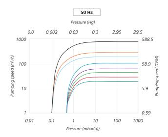
\*With gas ballast closed. Pump performance is measured at the inlet pressure and 20°C. Accuracy is +/- 10%.
