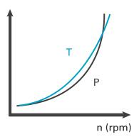
A compressor is a **constant torque** application. Here the input power/input current varies directly with the speed. The average current of drives used in constant torque applications is higher than for quadratic loads. Those applications are referred to as heavy duty.
