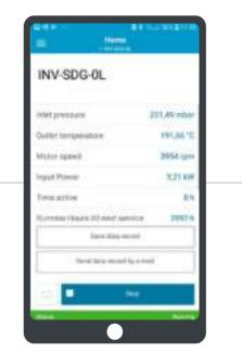
With the VSD<sup>+</sup> app, you also have live visualizations of the actual performance and settings. You can monitor details such as inlet pressure, rotor speed, running hours and service intervals.
